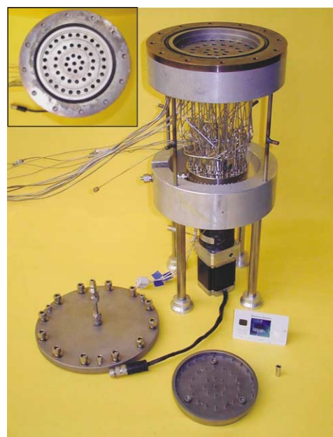
Fig. 1. Schematic drawing of a cross section of the 49-parallel channel reactor (a) and photograph of the reactor (b) with open lid, distribution plate from side and top view (size comparison: credit card).
